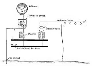
FIG. 110. Voltmeter and switches arranged for detecting "grounds" in electric circuits.
